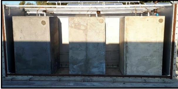
**Figure 2** Picture of the IMCB-ODE experimental device before immersion, containing 3 low-pH concrete blocks.
