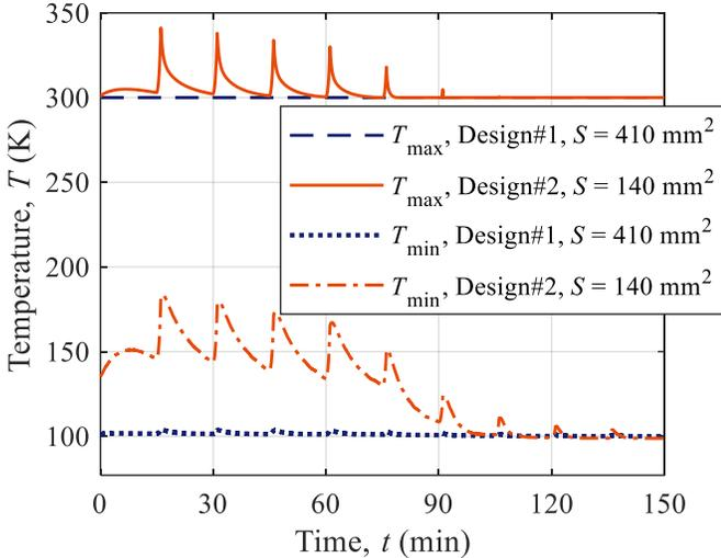
Fig. 10. Maximum ( $T_{\max}$ ) and minimum temperatures ( $T_{\min}$ ) over time for both designs. These temperatures are calculated for the part of the terminations that is not immersed in liquid nitrogen.
