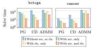
20 logarithmically spaced values of  $\lambda$  to span different working regimes and we report the overall solution time. We observe an acceleration factor up to three orders of magnitude when implementing both screening and relaxing tests compared to a vanilla implementation of PG, CD and ADMM, which assesses the interest for the presented "Screen & Relax" strategy.
