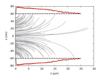
FIG. 11: Simulated ion trajectories (gray curves) through a 25  $\mu$ m long nanocapillary of inner radius of 60 nm, as indicated by the black dashed line. The red curves indicate the accumulated charge in arbitrary units at the inner interface.
