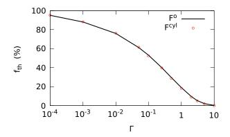
FIG. 4: Theoretical transmitted fraction  $f_{\rm th}$  (in percentage) as a function of the dimensionless parameter  $\Gamma$  defined by Eq. 9 in the case of a uniform, divergence-less ion beam aligned with the capillary axis. Full black line has been computed using  $F_{\rm im}^{\circ}$  while the red circles were obtained with  $F_{\rm im}^{\rm cyl} = F_{\rm im}^{\circ} \times h_{\varepsilon_T}$  and  $\varepsilon_T = 2$ .
