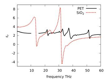
FIG. 8: Real part of the dielectric response function of SiO<sub>2</sub> (red dashed line) and PET (black full line) extracted from [27] and [22, 28, 29] respectively.
