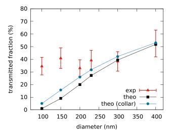
FIG. 6: Comparison between experimentally transmitted fractions (red triangles) extracted from [15, 16] and our theoretically transmitted fractions as a function of the capillary diameter  $2R_i$ . Experimental data are normalized such that fractions coincides for capillaries with 400 nm diameter. Filled blue circles give the theoretically transmitted fractions in the case where the inlet and outlet diameters include a 20 nm collar, filled black squares are evaluated without collar.
