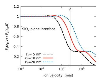
FIG. 9: Normalized image charge force  $F_z(z_p, v)/F_x(z_p, 0)$  as a function of the ion velocity v, for 3 different distances  $z_p$  from the SiO<sub>2</sub> interface,  $z_p = 5{,}10$  and 20 nm. The arrow indicates the velocity of 7 keV Ne<sup>7+</sup> ions as used by Sahana et al. [4].
