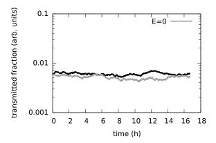
FIG. 1: Simulated transmitted beam fractions (black curve) through an insulating nano-capillary. The gray curve, for which the electric filed due to deposited charges was removed, has been added for comparison.
