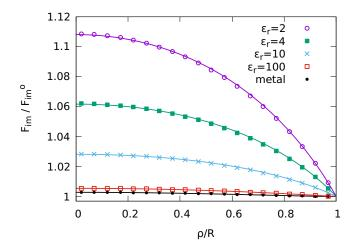
FIG. 2: Ratio  $F_{\rm im}$  /  $F_{\rm im}^0$  as a function of  $\rho/R$  for various  $\varepsilon_r$ . The label "metal" stands for a perfectly conducting interface. The full curves are the function  $h_{\varepsilon_r}(\rho/R)$  for  $\varepsilon_r=2,4,10,100$  and  $|\varepsilon_r|\to\infty$ .
