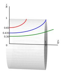
FIG. 3: Trajectories for 3 different initial values of  $\varrho_0$  in the case of  $\Gamma = 1$ . Only for  $\varrho_0^{\rm max} < 0.435$  are the ions transmitted, so that for  $\Gamma = 1$  the transmitted fraction  $f_{\rm th}$  equals  $\varrho^2 = 18.6\%$
