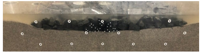
Figure 5. Post DMX03 image of the rock berm, side view
