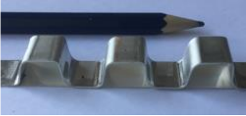
Fig. 3. REBCO tape with corrugated stabilizer (same width).
