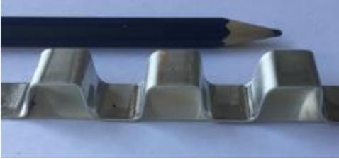
Fig. 3. REBCO tape with corrugated stabilizer (same width).
