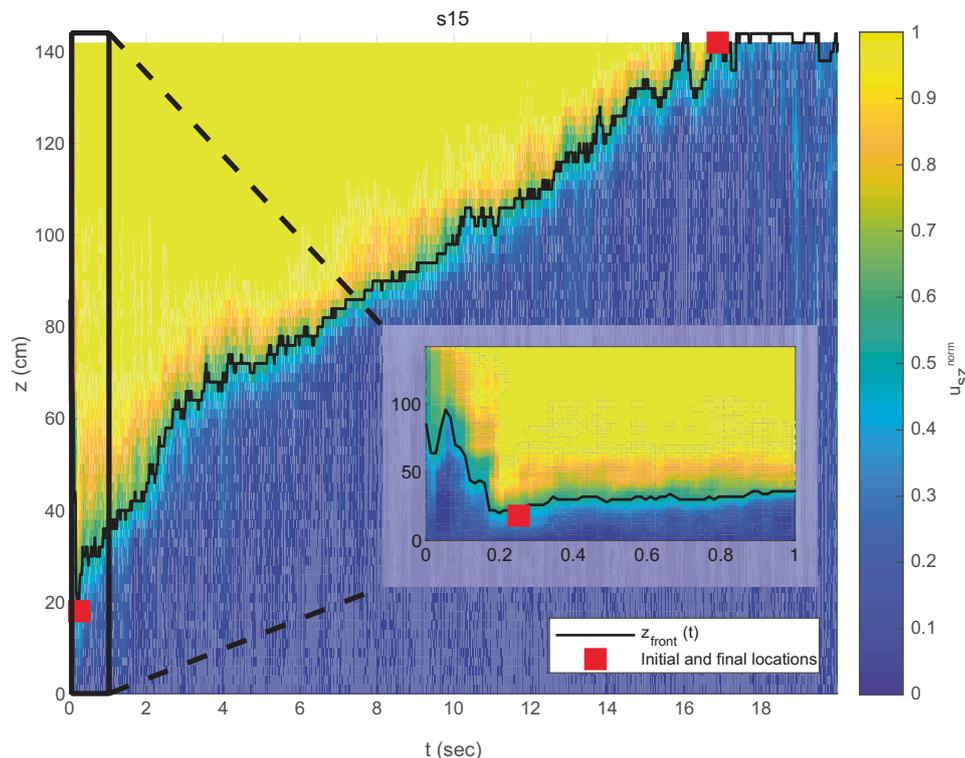
**Fig. 6 | Example of compaction front detection and calculation of the average front velocity  $u_{\text{front}}$ .** The vertical axis represents height above the bottom wall, and the horizontal axis is time. The color map shows the normalized averaged and smoothed vertical grain velocity,  $u_{\text{sz}}^{\text{norm}}$ . The black curve depicts the inferred front location ( $z_{\text{front}}(t)$ ). The front velocity is calculated as the average slope of the black
