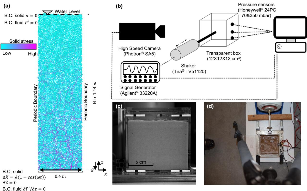
**Fig. 5 | Numerical and experimental setups.** **a** Schematics of the simulations setup and boundary conditions. **b** Schematics of the experimental setup. **c** The front face of the experiment box (a frame from the high-speed camera used for velocimetry).
