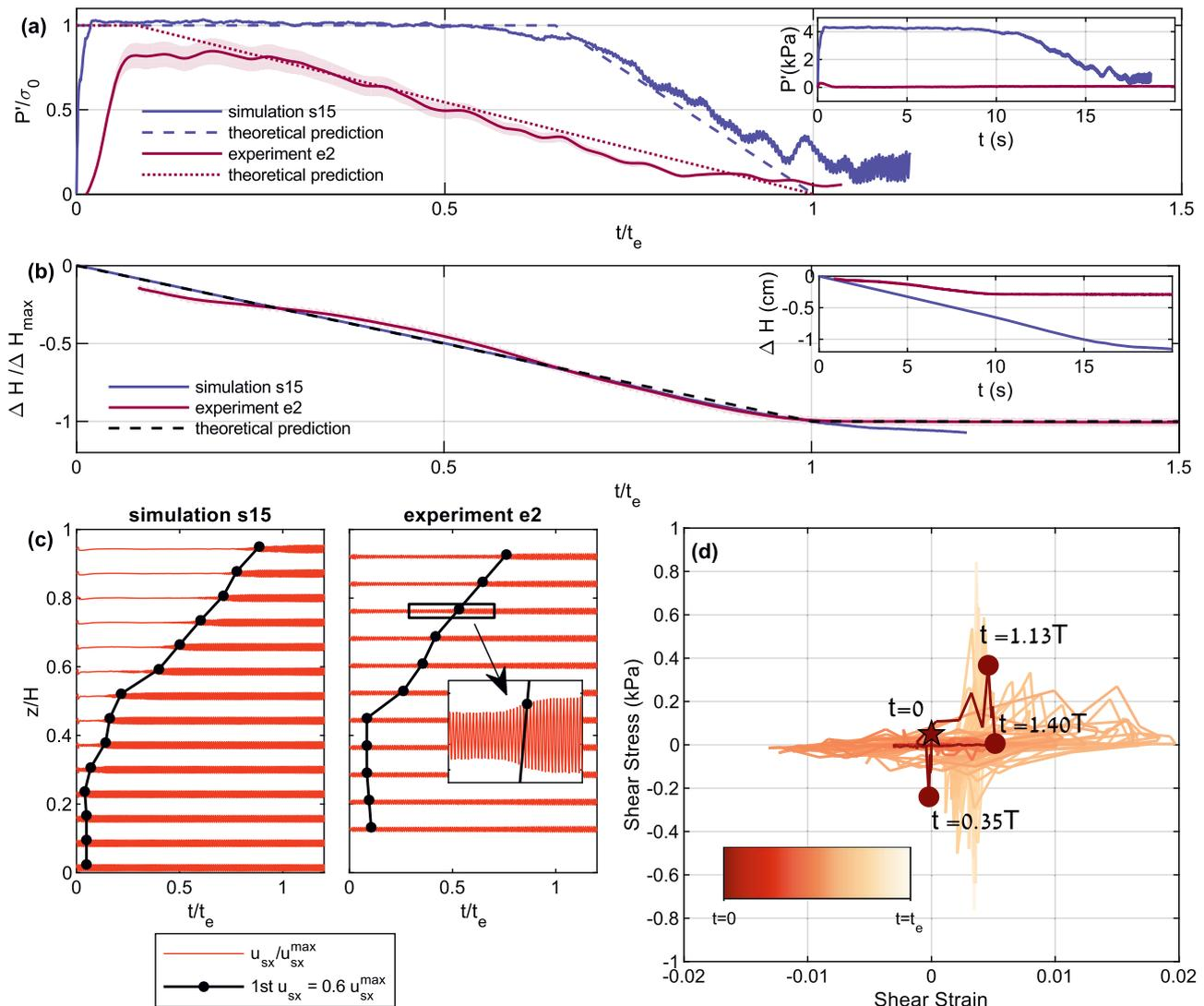
**Fig. 2 | Liquefaction indicators in drained simulations and experiments.**
