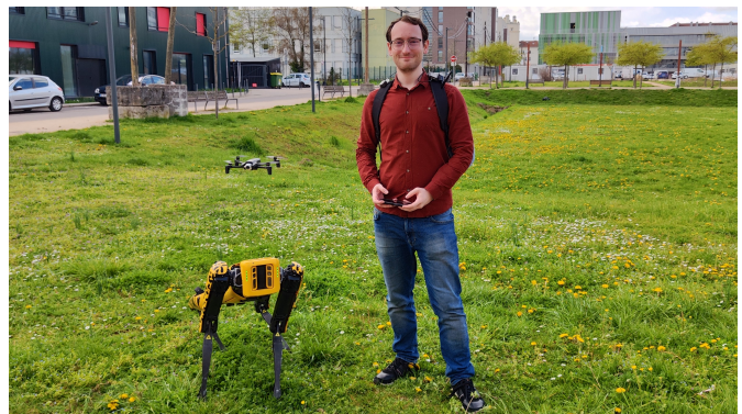
Fig. 1. An HMAS composed of a ground quadruped robot (Spot), an aerial drone currently flying (Anafi), and a human operator equipped with sensors on a backpack. All agents and humans have RTK GPS to locate themselves in an outdoor environment.
