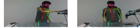
(a) MwoGR: Press robot to start (b) MwGR: The robot recognizes G 7 to start
