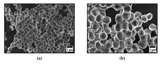
Figure 1. SEM (scanning electron microscopy) images of the chosen alumina powders with average particle sizes of around (a) 0.7  $\mu m$  and (b) 1.3  $\mu m$  respectively.
