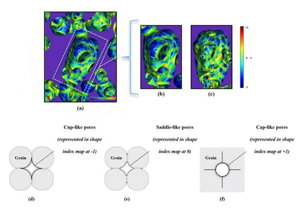
Figure 16. Snapshots of the (a) 3D rendering of the shape index values of the evolving pore network, for the in-situ observation of Al 1.3 $\mu$ m after (b) 1 hour and (c) 5 hours of sintering at 1500°C respectively. Representation of pore evolution during the sintering process from (d) the initial cup-like pores to (f) the final cap-like pores, including an (e) intermediate transition step with saddle-like pores.
