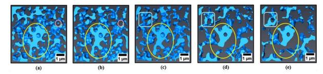
Figure 9. Follow-up of the mechanisms occurring in the pore network for the in-situ observation of Al 0.7 $\mu$ m after (a) 20 min, (b) 30 min, (c) 45 min, (d) 1 hour and (e) 2 hours of sintering at 1500°C respectively.
