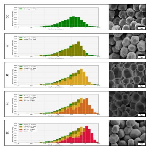
Figure 11. Evolution of surface smoothness for the in-situ X-ray nano-CT observation of Al 1.3 $\mu$ m at (a) the green state, and after (b) 20 mins, (c) 1 hour, (d) 3 hours and (d) 5 hours of sintering at 1500°C respectively, with their corresponding SEM observations.
