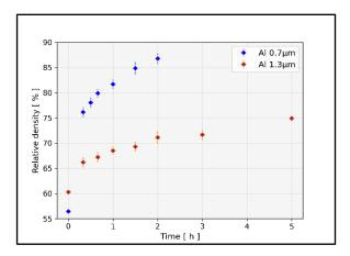
Figure 5. Relative densities as a function of time for the sintered samples of Al 0.7 $\mu$ m and Al 1.3 $\mu$ m.
