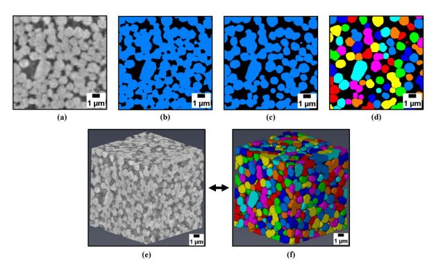
Figure 4. Steps of image improvement leading to segmentation, showing different preprocessing operations for a (a) raw image data - (b) binarization, (c) morphological opening and (d) watershed segmentation followed by labelling of grains. 3D rendering of the initial volume and (f) its final segmented state.
