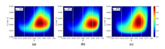
Figure 15. Pore curvature maps for the in-situ observation of Al 0.7μm after (a) 10min, (b) 1 hour and (c) 2 hours of sintering at 1500°C respectively.
