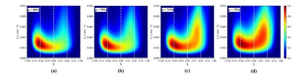
Figure 14. Pore curvature maps for the in-situ observation of Al 1.3µm after (a) 1 hour, (a) 2 hours, (c) 3 hours and (d) 5 hours of sintering at 1500°C respectively.
