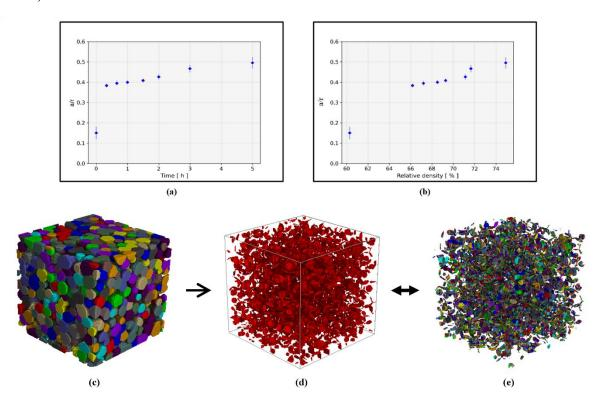
Figure 12. (a) Growth of the average inter-particle neck ratio (a) over time and (b) versus density for the alumina Al 1.3 $\mu$ m. Close-up of (c) cropped segmented section of alumina Al 1.3 $\mu$ m and its corresponding neck morphology, (d) prior to segmentation and (e) post-segmentation.
