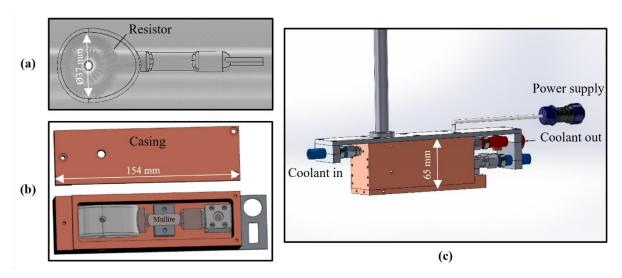
Figure 2. (a) Internal design of the furnace resistor, imaged from a laboratory tomography source (*EasyTom XL by RX-Solutions*), (b) components of the furnace system inside the casing, assembled together to set up the (c) cooling system.
