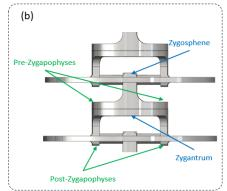
**Figure 3.** (a) Biological snake vertebrae (*Natrix natrix*). (b) Equivalent snake robot flexible vertebrae.
