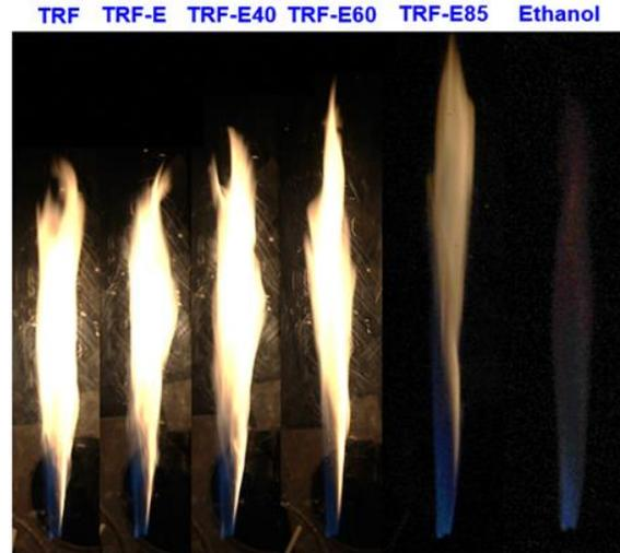
Fig.3. Pictures of the 6 TRF-Ethanol (0-100%) flames with constant LVH
