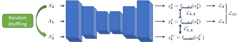
Figure 2: Schema of the self-supervised training of the back-bone. The three different losses are alternatively used to modulate the model weights: the deep clustering loss \mathcal{L}_{DC} , the temporal consistency loss \mathcal{L}_{1,2} (with attractive arrows) and the contrastive loss \mathcal{L}'_{1,2} (with repulsive arrows).
