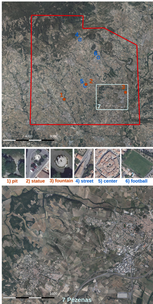
Fig. 7. Overview of the regions of interest used for the quality estimation considering tie point accuracy and reprojection error (1–3), accuracy estimation with multi-temporal DSMs (4–6), and qualitative use of the DSMs for change detection analysis close to the city Pézenas (7).
