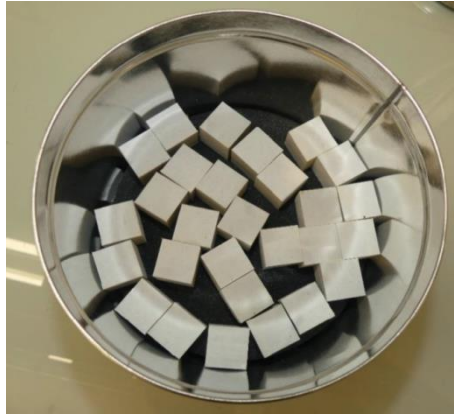
Figure 9: Small BC samples used to study the regression rate in the HPV
