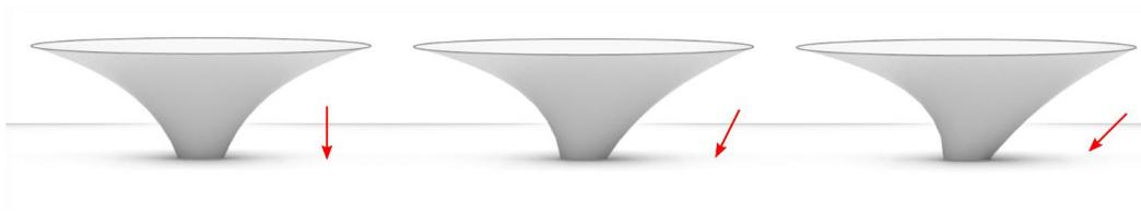
**Figure 13: i-minimal membranes constructed on the same boundary, but with different isotropic directions**
