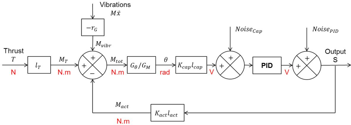
Figure 4: Block diagram of the nulled dual pendulum thrust stand.
