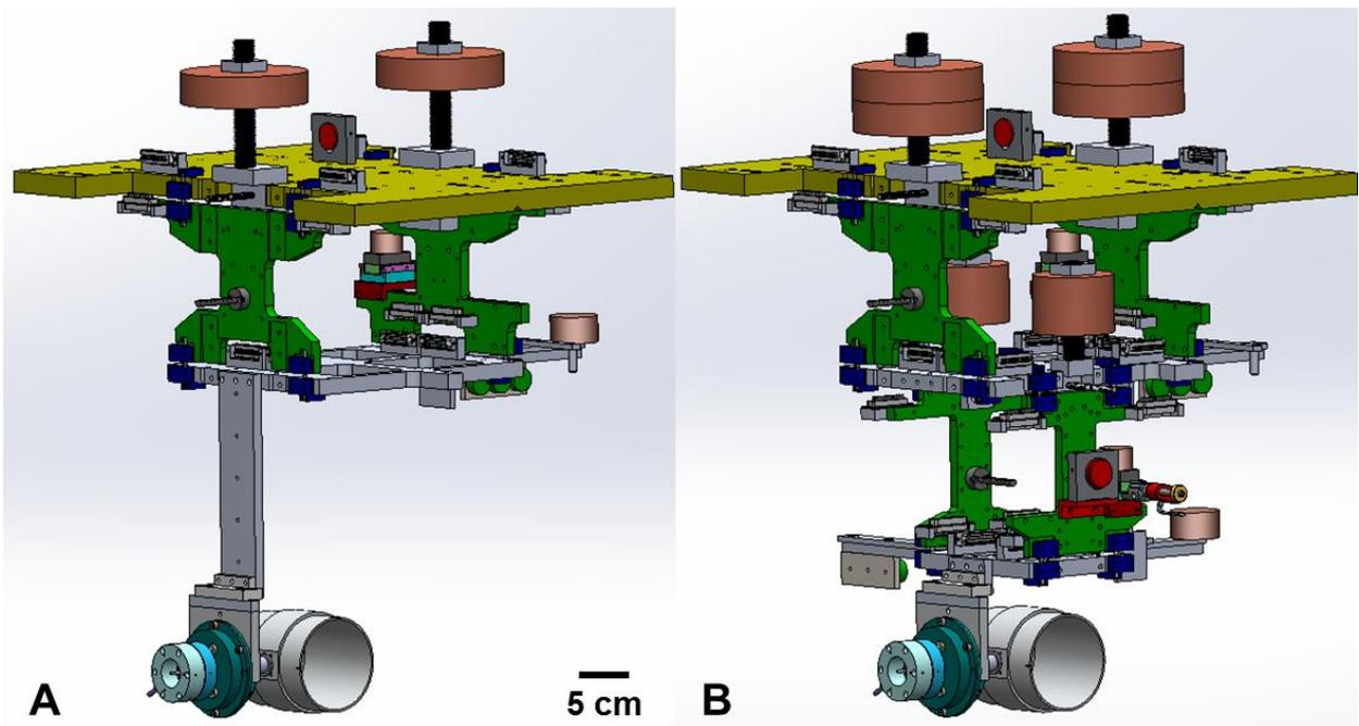
Figure 5: CAD model of the thrust stand concept. A) 1-axis dual pendulum TS. B) 2-axis TS. Yellow: Fixed platform. Blue: Be-Cu strips and fastening. Green: Arms with counterweights above the fixed pivots, one accelerometer per stage and one actuator. The calibration comb is also visible. Grey: Moving platform with capacitive sensor target and magnets for the damping and the actuation. The ECR thruster is at the bottom.
