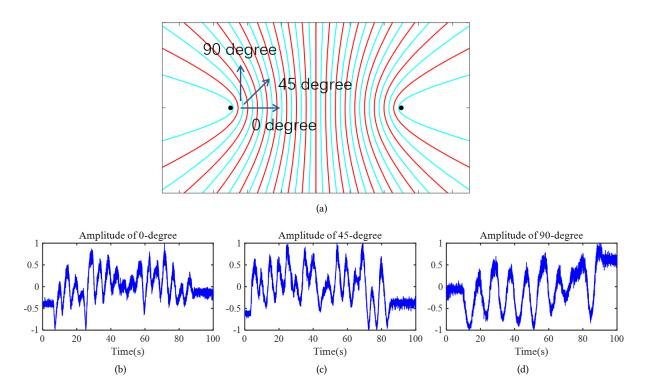
Fig. 7. Dynamic Fresnel zone experimental settings (up) and results (down): (b) 0-degree, (c) 45-degree, (d) 90-degree.
