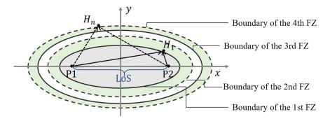
Fig. 2. Geometry of the Fresnel Zone
