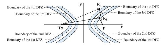
Fig. 4. Geometry of the Dynamic Fresnel Zone
