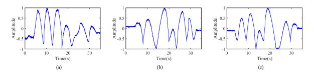
Fig. 8. Received CSI amplitude when the distance between surrounding subject and transmitter is: (a) 2.4m, (b) 3.6m, (c) 4.2m.
