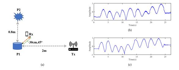
Fig. 11. Experiment setup in a real-life scenario (a), CSI amplitude obtain when there is only one surrounding subject (P1) (b) and two neighboring surrounding subjects P1 and P2.
