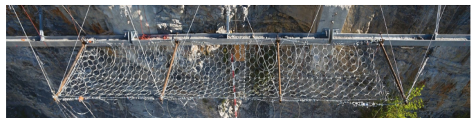
Figure 14: Front view of the tested rockfall barrier prototype (by courtesy of national project C2ROP)
