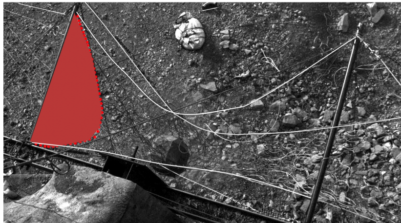
Figure 20. Side hole in the barrier after the lateral impact during the second campaign.
