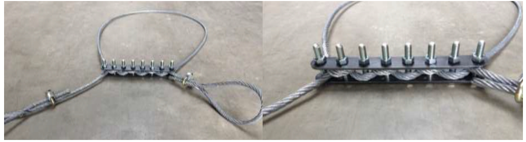
Figure 3. Image of the so-called snake brake provided by NGE foundations: it is made of two steel plates connected by a series of bolts through which a cable is braided at both end of the loop (by courtesy NGE foundations).
