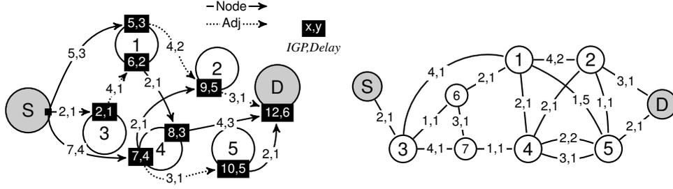
Figure 4. A raw network (at the right), and its resulting meta-DAG of *all* the segment lists from S towards node D having distance (12, 6).
