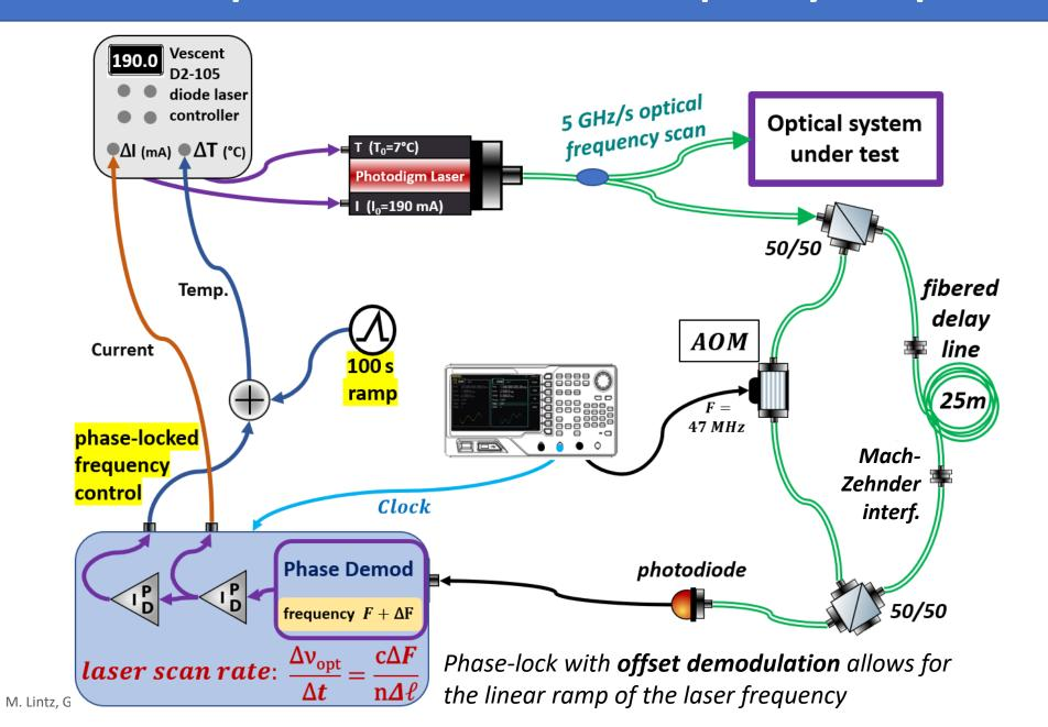
2nm-span optical frequencyscanned laser source
