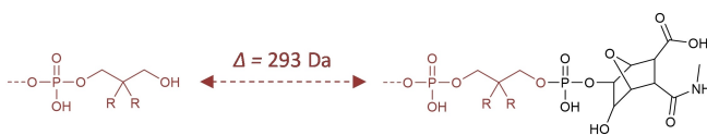
Figure 4. Different types of \alpha -chain-ends observed for the formed polymers after cleavage from commercial UnySupport. Left: targeted hydroxyl chain-ends. Right: chains containing a residual group due to incomplete dephosphorylation.
