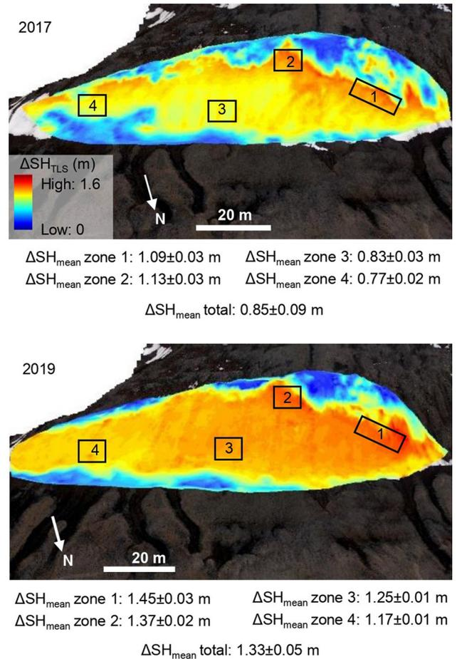
**Figure 7.** Maps of the total surface ablation ( $\Delta SH_{TLS}$  in m) during the study periods 2017 and 2019 based on daily terrestrial laser scan (TLS) surveys of snow/ice surface position. The black boxes represent the averaging area used to highlight the spatial variability of the ablation. Mean ( $\pm$ std. dev.) values for the whole ice patch and each zone are presented below each panel.
