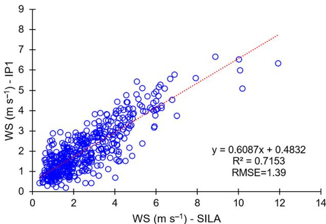
**Figure 15.** Correlation between the hourly average wind speed derived from SILA measurements adjusted using Eqn (A1) for a 2 m-height level at the SILA station from time series provided by the anemometer at 10 m and by the AWS on IP1 during the study period 2019.
