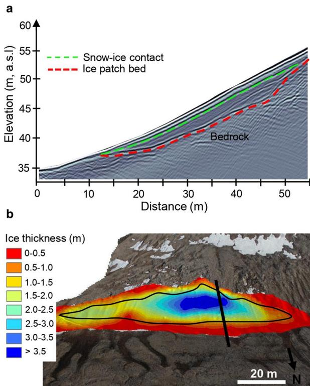
**Figure 6.** (a) 2D visualization of a GPR profile made in the central part of the ice patch in 2019 using 100 MHz antennas (the track is represented by the black line in (b)). (b) Interpolated map of the ice thickness based on the series of GPR tracks made in July 2019 (see Fig. 2 for all GPR tracks location). The black line in (b) delimits the contour of the ice body at the end of summer 2016.
