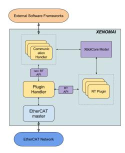
**Figure 1.** The diagram shows *XBotCore* components interactions: an EtherCAT master RT thread communicates with the EtherCAT slaves and with the Plugin handler RT thread which schedules execution of a set of RT plugins. The Communication Handlers non-RT threads allow interfacing with non-RT external Software Frameworks
