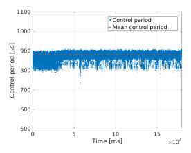
**Figure 3.** WALK-MAN control period during manipulation actions: XBotCore assures always a control period below  $1000\mu s$
