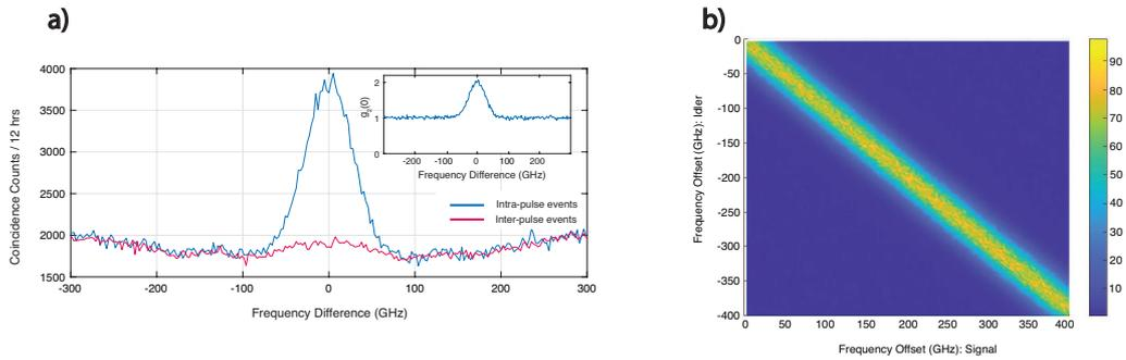
**Figure 2. a)** Second-order auto-correlation function of the signal field, as function of frequency difference between the spectral components. **b)** Joint spectral intensity (JSI) and the CAR versus the signal and idler frequency offset from the SPDC degeneracy point.
