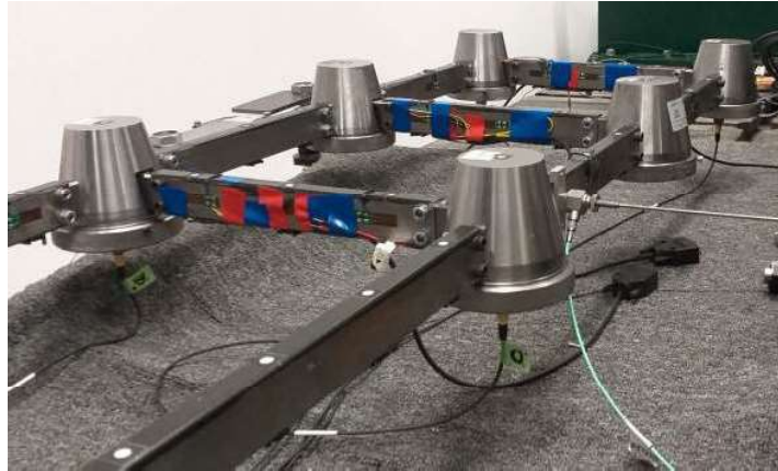
Figure 1: Demonstration stand with six lockable joints
