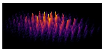
Fig. 1. Measured FROG (Frequency-Resolved Optical Gating) trace of a typical multiple pulse pattern generated by the on-chip IMZ cascade system.
