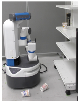
Fig. 9: Demonstration setup emulating a convenience store shelf, comprises a Fetch Robot, a shelf and three types of Noodle Cups. In the proposed scenario, two cups have fallen on the ground, in an unknown pose, due to a customer action.
