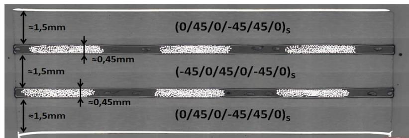
**Figure 3.** Cross-section of multi-layered composite functional structure.
