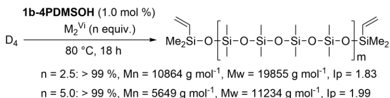
Fig. 3. Fully converted anionic ring-opening polymerizations (ROP) of D 4 . (A) Study of the effects of phosphonium cations on the ROP of D 4 with different initiators 1-xROH . (B) Study of polymer size control by end capping agent (M 2 Vi ) in the ROP of D 4 with the phosphonium benzyloxy initiator ( 1b-4BnOH ). (C) Synthesis of PDMS-based initiator 1b-4PDMSOH and its tests for the full ROPs of D 4 in the presence of M 2 Vi .
