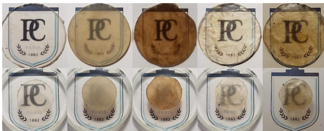
Figure S15. Photographs of samples just above ESPCI logo (top row) and at 1 cm height (bottom row). From left to right: S , Ext<75 \mu\text{m} , Ext>75 \mu\text{m} , Vit sol and BisBE Vit . Yellowish color comes from H that is yellow and possibly from the degradation products of antioxidant used (Irganox 1010). [S11]
