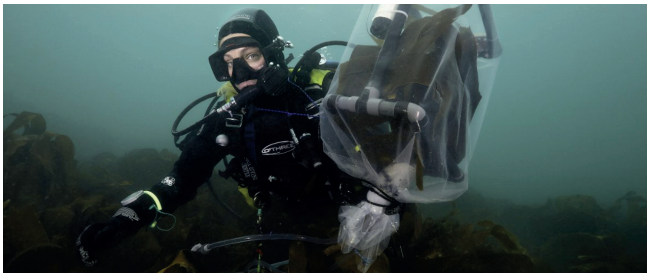
Figure 4. In situ photorespirometry for direct measurement of primary production in a kelp forest in the vicinity of Roscoff operated by Lydia White (credit Wilfried Thomas SBR).
