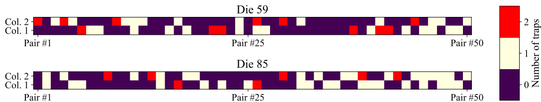
Fig. 13. Cartography of the detected RTN traps within the columns of the test structure corresponding to the W = 0.08 \mu\text{m} , L = 0.03 \mu\text{m} devices, for two different dies, extracted at V_g = 1 \text{ V} .
