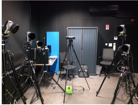
Fig. 4. Motion capture and Kinect setup. Point of view of the captured subject.
