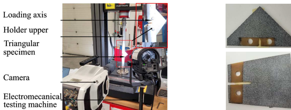
Fig. 1 – Experimental set-up under quasi-static loading.
