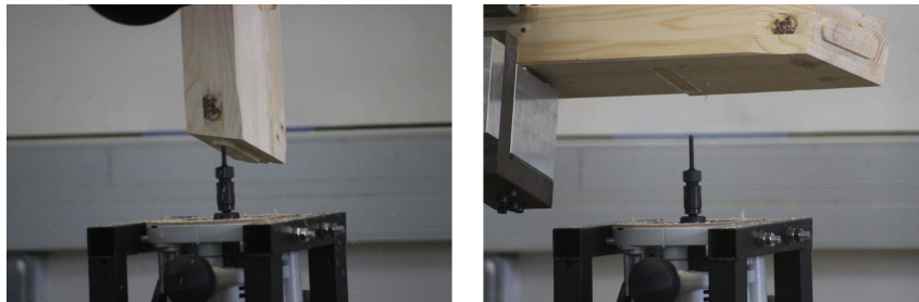
Fig. 15 Hole-drilling step: longitudinal and transversal pilot holes.
