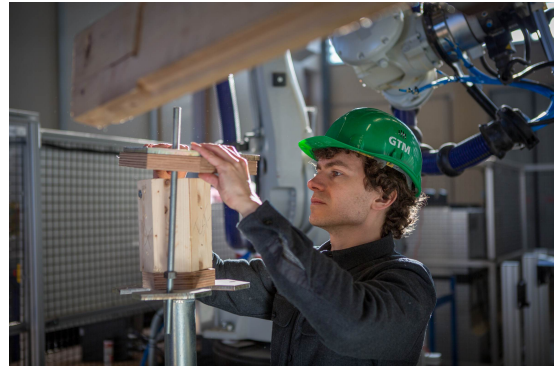
(a) Node assembly on a fixed support
