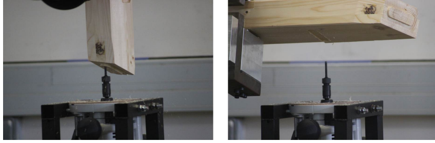
Fig. 15 Hole-drilling step: longitudinal and transversal pilot holes.
