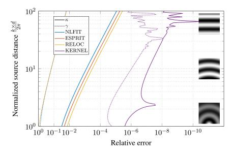
Figure 5: Wavevector estimation bias associated to cylindrical wave field. Effect of the distance d to the source  $\underline{x}_0$  in the estimation of the isotropic wavenumber  $k = \kappa (1 - i \gamma) = \frac{6\pi}{L} (1 - 0.05 i)$ .
