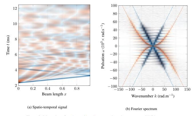
Figure 3: Dispersion of torsion and bending waves in an homogeneous PVC beam
