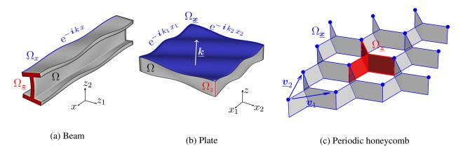
Figure 1: Typical waveguides
