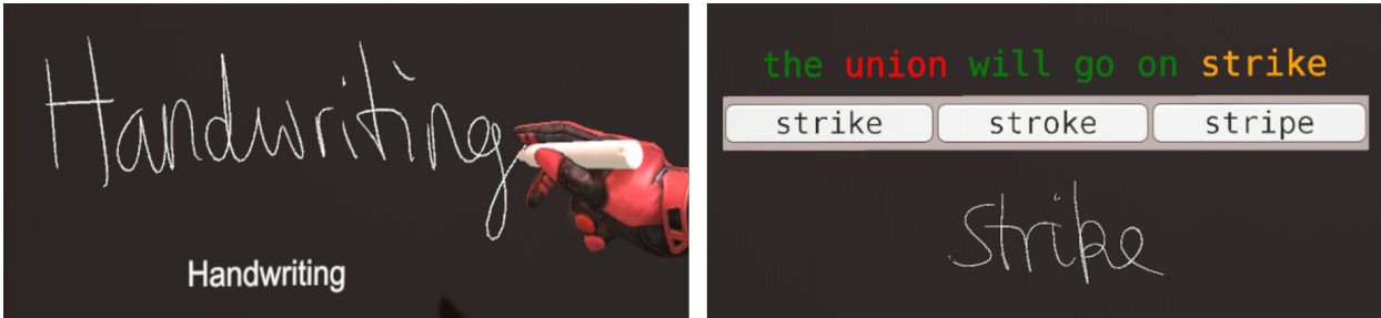
Fig. 1: The user can write words by hand on a board in the virtual environment. Handwriting recognition technology converts the handwritten word into usable text data (left). During the user study, participants are presented with phrases they have to write one word at a time (right). The yellow word is the selected word. Green words are correctly recognized and red words are not. Users are presented with multiple recognition results they can choose from.
