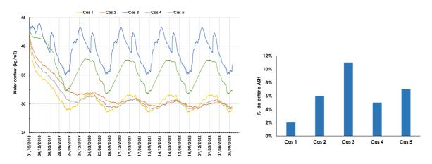
Figure 1. (a) Total water content of the wall with different coatings (b) Ash criteria of the wall with different coatings
