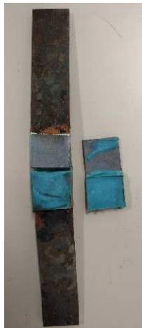
Figure 13. Double lap shear specimen after being tested.
