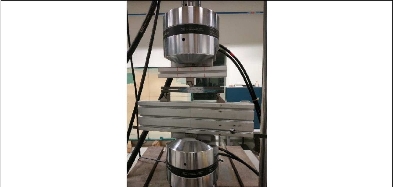
Figure 14. End Notched Flexure Tests.
