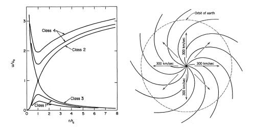
Figure 3: Parker's analytical solutions showing the solar wind velocity profile,  $u/u_c$ , versus the radial distance from the Sun,  $r/r_C$  (left panel, the subscript C indicating the coronal Alfvénic critical point, see Hundhausen, 1972), and a schematics of the interplanetary magnetic field spiral. Figure adapted from Hundhausen (1972).
