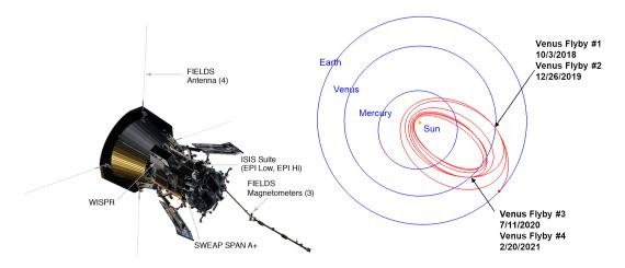
Figure 49: Left: rendering of the Parker Solar Probe, with the indication of the paylod location (source: JPL, available at http://parkersolarprobe.jhuapl.edu/index.php). Right: a graphical view of the typical PSP orbits (source: NASA, available at https://blogs.nasa.gov/parkersolarprobe/2019/12/23/parker-solar-probe-heads-toward-second-venus-flyby).
