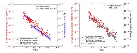
Figure 5: Radial profile of energy injection rate,  $\varepsilon$ , as measured by Parker Solar Probe during its first perihelion, compared with the estimated plasma heating rate, H (left panel), and with the estimated energy reservoir from the low-frequency fluctuations, S (right panel). Full and empty symbols refer to the inbound and outbound portion of the spacecraft orbit, respectively. Figure adapted from Wu et al. (2022a).
