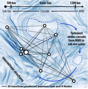
Figure 107: Top panel: illustration of the NASA/Helioswarm 9 spacecraft configuration. Credits: UNH EOS (available at https://www.unh.edu/unhtoday/2022/02/solar-windfall). Bottom panel: a rendering of the mission concept, with possible 36 baselines covering scales Figure from https://www.lpl.arizona.edu/missions/helioswarm.
