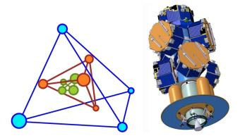
Figure 106: Left panel: the ESA/Cross-Scale mission proposal logo, representing the nested-triple tetrahedron spacecraft configuration. Figure from (Schwartz et al., 2009). Right panel: a rendering of the mission launching configuration, with the 12 spacecraft stacked on a bus. Figure from the ESA Cross-Scale Assessment Study Report (SRE-2009-1), Publication date: 01 December 2009, available at https://sci.esa.int/documents/34697/35949/1567257732515-SRE-2009-1\_Cross-Scale21.pdf.
