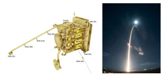
Figure 50: Left: rendering of the Solar Orbiter spacecraft, with labels indicating the payload (source: IRF, available at https://www.irf.se/sv/irf-i-rymden/solar-orbiter). Right: a picture of the Solar Orbiter launch from the Cape Canaveral site (source: ESA, available at https://www.esa.int/Science\_Exploration/Space\_Science/Solar\_Orbiter/Liftoff\_for\_Solar\_Orbiter\_ESA\_s\_mission\_to\_face\_the\_Sun\_up\_close).
