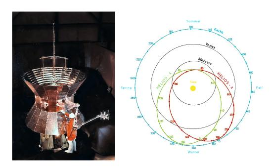
Figure 44: Left panel: a picture of the Helios 2 spacecraft during testing. Right panel: the orbit of Helios 1 and Helios 2. Credits: NASA/Max Plank Institute. Available at: left: https://en.wikipedia.org/wiki/Helios\_(spacecraft); right: https://heasarc.gsfc.nasa.gov/docs/heasarc/missions/images/helios2\_images.html
