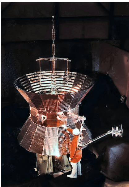
Figure 44: Left panel: a picture of the Helios 2 spacecraft during testing. Right panel: the orbit of Helios 1 and Helios 2. Credits: NASA/Max Plank Institute. Available at: left: https://en.wikipedia.org/wiki/Helios_(spacecraft) ; right: https://heasarc.gsfc.nasa.gov/docs/heasarc/missions/images/helios2_images.html
