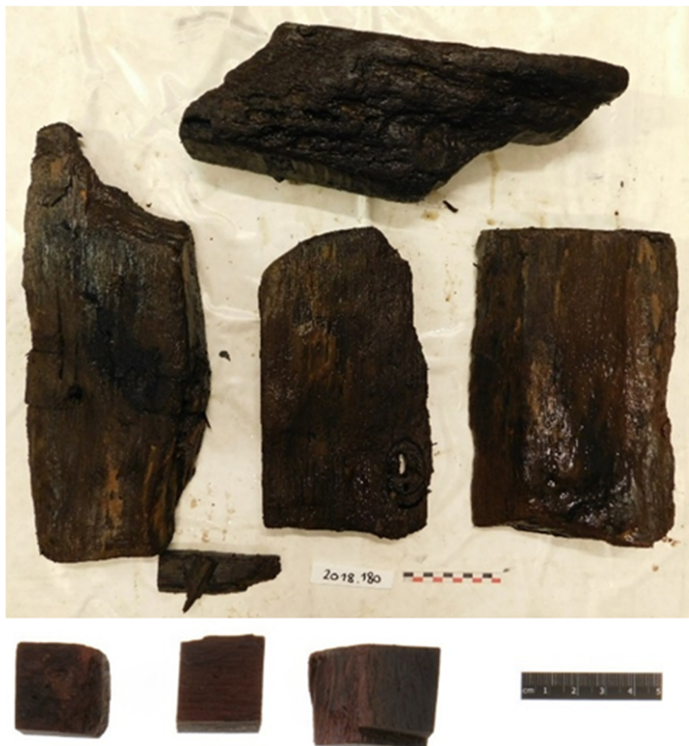
Figure 1. Waterlogged archaeological wood from the archaeological site “Saint-Lupien”, Rezé, Nantes (FRANCE), and below, samples after cutting (3 × 3 × 3 cm) used for extraction treatments.
