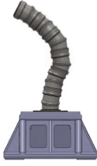
FIGURE 2. ROBOT NB-R1 FORMED OF SIX NB-MODULES
