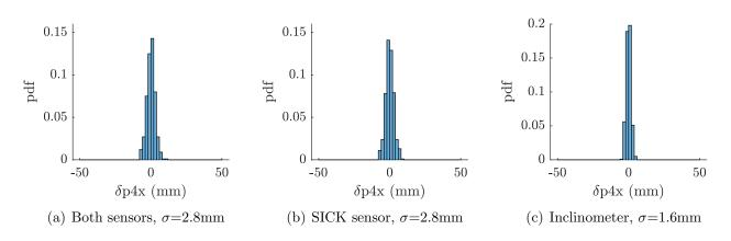
Figure 21: Identification error results in the x-coordinates of the 4th MP position vector when 50 poses are used, comparison of sensor effects
