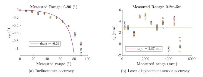
Figure 9: WitMotion BWT61CL inclinometer and SICK DT50-2 laser displacement sensor accuracy curve fitting
