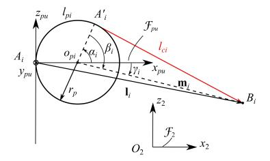
Figure 4: Parameterization of the *i*th pulley
