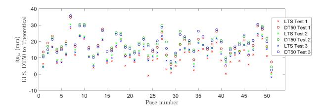
Figure 27: Differences between measured and desired MP height
