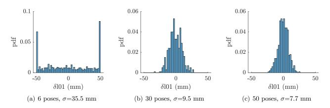
Figure 16: Identification error results of the initial length in the 1st cable, with different numbers of measurement poses and  $\sigma$  values
