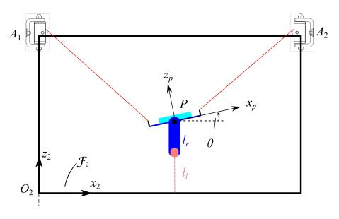
Figure 2: CDPR geometry inside  $\mathcal{F}_2$
