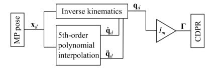
Figure 13: CDPR position control scheme
