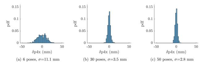
Figure 17: Identification error results of the x-coordinates of the 4th MP position vector, with different numbers of measurement poses and  $\sigma$  values
