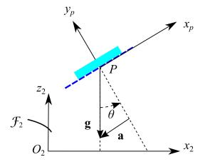
Figure 8: Inclinometer working principle
