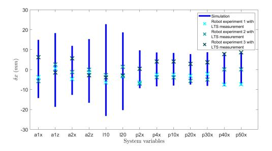
Figure 32: Calibrated system variable identification errors
