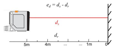
Figure 10: Laser displacement sensor accuracy test schematic
