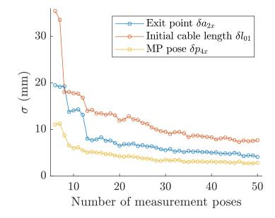
Figure 14: The standard deviation results of 3 examples of the system variables
