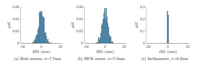
Figure 20: Identification error results in the initial cable length of the 1st cable when 50 poses are used, comparison of sensor effects
