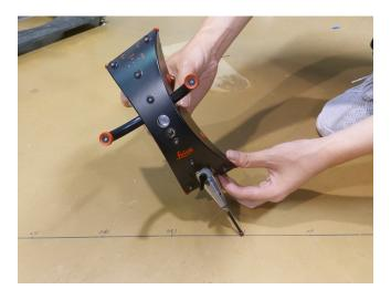
Figure 11: Floor elevation measurement with laser tracker T-probe
