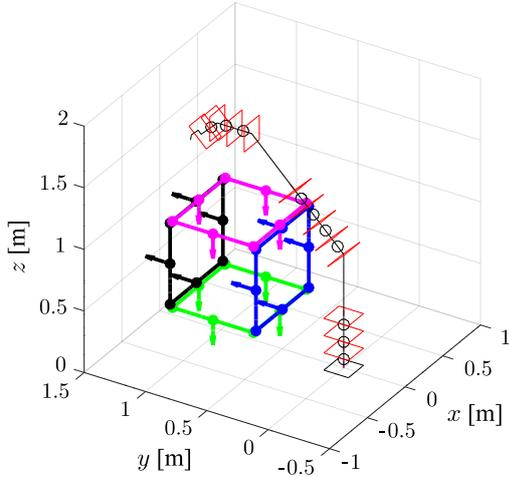
Figure 4: The four paths used in the optimization process and a version of Nimbl'bot robot of size:  $l_1 = 0.5$  m,  $l_2 = 0.5$  m,  $\beta_1 = \pi/4$ ,  $\beta_2 = \pi/4$ ,  $\beta_3 = \pi/4$ ,  $l_t = 0.1$  m,  $\beta_t = \pi/4$ .
