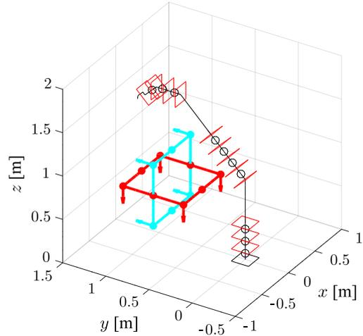
Figure 5: The two paths used to validate the designs obtained from the optimization process and a version of Nimbl'bot robot of size:  $l_1 = 0.5$  m,  $l_2 = 0.5$  m,  $\beta_1 = \pi/4$ ,  $\beta_2 = \pi/4$ ,  $\beta_3 = \pi/4$ .
